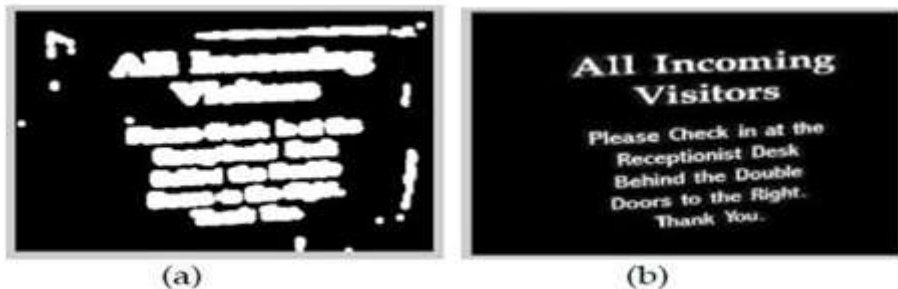
Fig.5. (a) Image after morphological operations, (b) Output image after segmentation.
